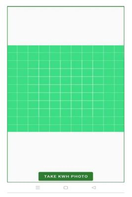
Click on the 'Take KWH Photo' (Single Phase) and take the proper photo of **KWH reading** in meter for Single Phase. For three phase meters need to take KWH and KVAH photos.
